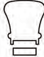
6010P HANDRAIL 1-1/4" PLOW 2-1/4" x 2-3/8" O, M, POP, KA, KP
