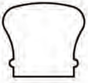
6210 HANDRAIL (NO PLOW) 2-5/8" x 2-3/8" O, M, POP, KA, KP
