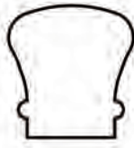
6010 HANDRAIL (NO PLOW) 2-1/4" x 2-3/8" O, M, POP, KA, KP
