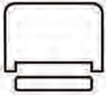
6770P1 HANDRAIL 1-3/4" PLOW 2-1/4" x 1-5/8" O, M, POP, KA, KP
