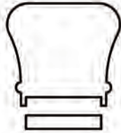
6210P HANDRAIL 1-3/4" PLOW 2-5/8" x 2-3/8" O, M, POP, KA, KP
