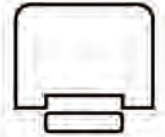
6770P HANDRAIL 1-1/4" PLOW 2-1/4" x 1-5/8" O, M, POP, KA, KP
